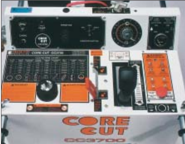
CC3700 Control Panel
