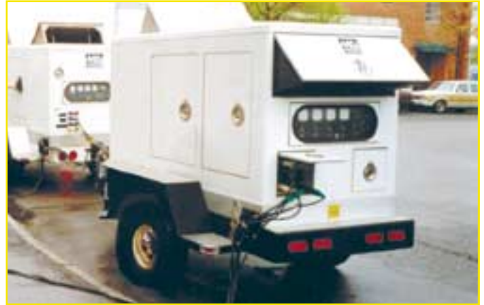
Crawford Studio Generator (EGS500C)
