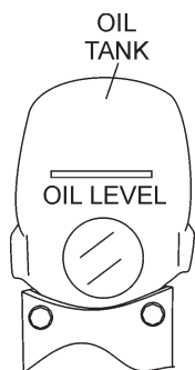
Figure 9. Oil Tank (Front View)
