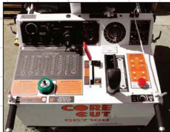
CC7100 Control Panel with drive lever, power raise/lower buttons and gauges
